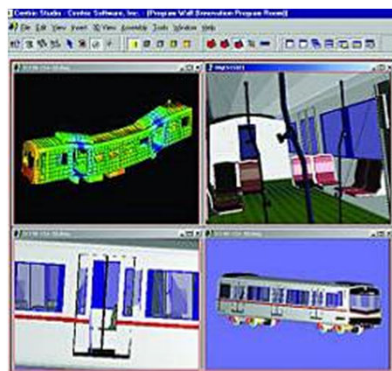
A Siemens subway car is virtually modeled during the conceptual design phase.
